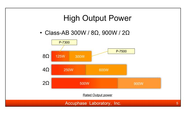
High power design provides the rated output power of  $300W/8\Omega$ ,  $600W/4\Omega$ , and  $900W/2\Omega$  that vastly exceeds conventional models, securing an overwhelming dynamic range.
