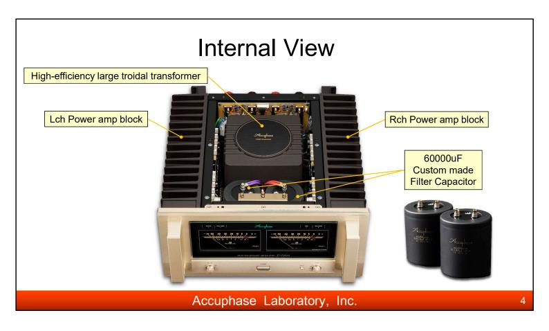
P-7500 has a mono-block construction.
