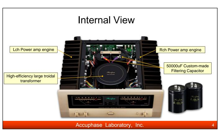
P-4600 has a mono-block construction.
