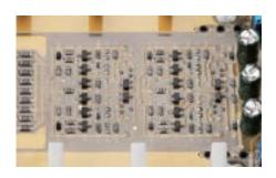
Current feedback principle provides excellent phase characteristics in high frequency range
