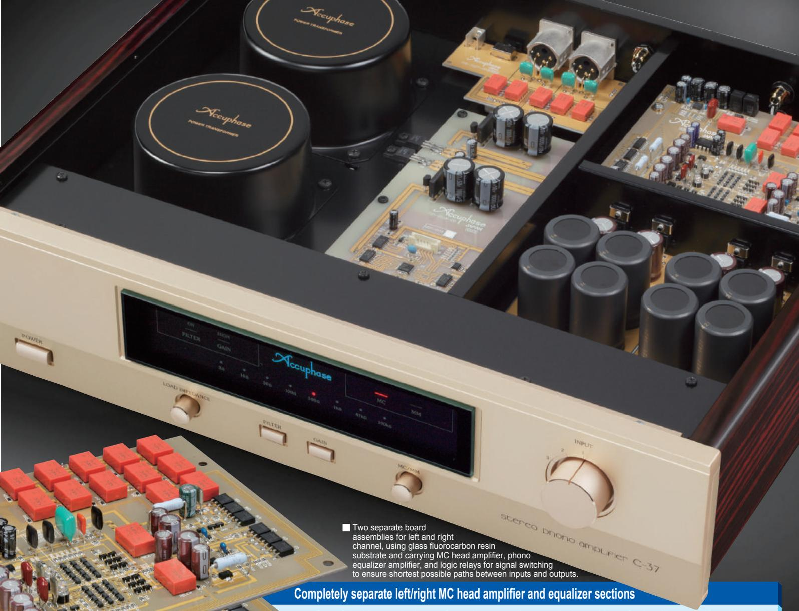
■ Two separate board assemblies for left and right channel, using glass fluorocarbon resin substrate and carrying MC head amplifier, phono equalizer amplifier, and logic relays for signal switching to ensure shortest possible paths between inputs and outputs.
