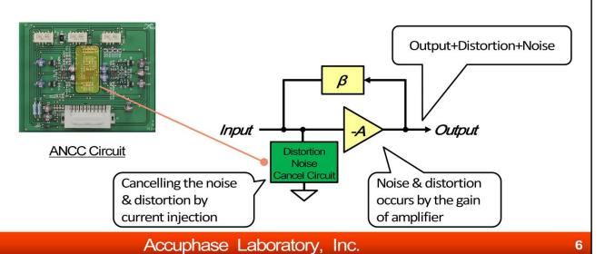
ANCC (Accuphase Noise and distortion Canceling Circuit) topology is installed in I-V Converter of AAVA.
