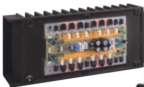
⑮ Power amplification section
