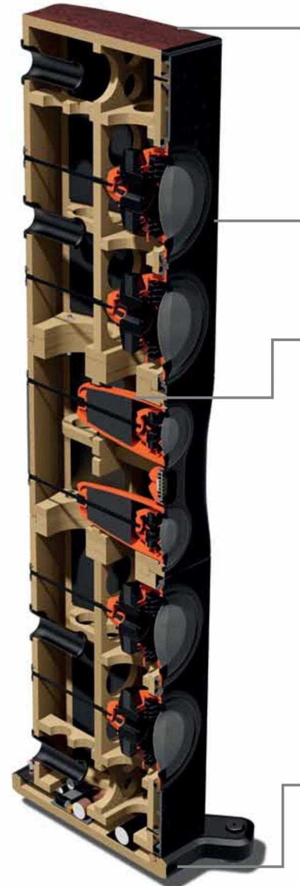
**CURVED AND BRACED CABINET CONSTRUCTION:** Curved surfaces are inherently stronger than flat surfaces, and since the internal sides are non-regular, standing wave formation is suppressed. New internal bracing structures have been developed to ensure the ultimate in structural integrity, and bitumastic damping material applied to all internal cabinet walls to ensure that all cabinet vibration is absorbed. Result: a supremely rigid, acoustically inert enclosure for natural, true-to-life fidelity.
