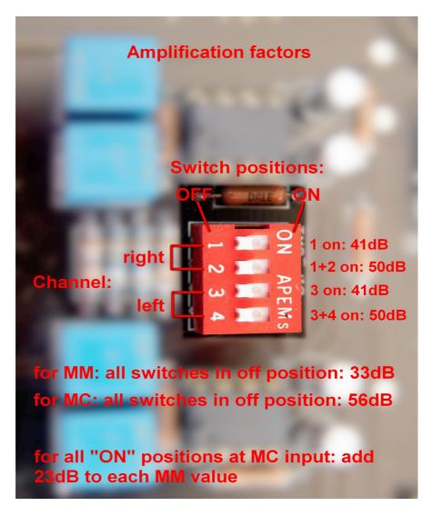
Switch No.1 and No.2 belong to the right channel and switch No.3 and No.4 belong to the left channel. Default position (delivery condition) is: all switches in position "off". That means, the basic amplification factor is for **MC input: 56dB** and for **MM input: 33dB**. Simply choose the desired amplification factor by pushing the respecting levers to the "on" position.
