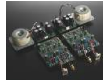
Left and right DAC circuit boards, and individual power supply units
