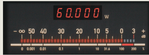
Digital power meter/bar graph meter
